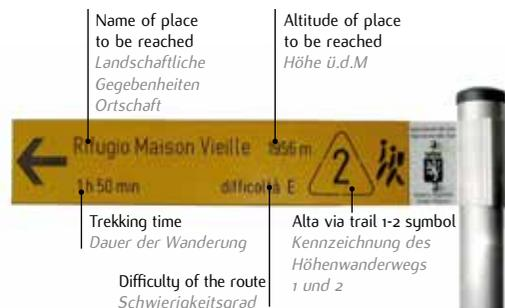
Vertical signpost consists of a vertical post (h 250 cm.), onto which are fixed yellow indication signs (size 10x 50cm.) showing the name of the place to be reached, with the relative altitude and trekking time (calculated for a moderately fit trekker with rucksack). The sign also indicates the difficulty of the route.
